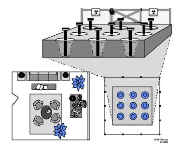
Figure M.2 Down-Hole Storage Array in Waste Broker Facility.
