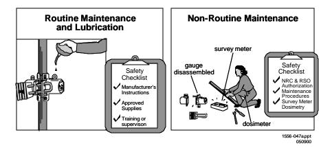
**Figure 8.12 Routine Maintenance and Lubrication.** *To ensure proper operation of the unit, licensees need to perform routine maintenance according to the manufacturer's (or distributor's) written instructions and recommendations.*
