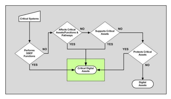
Figure 4 Evaluation process for identifying critical digital assets
