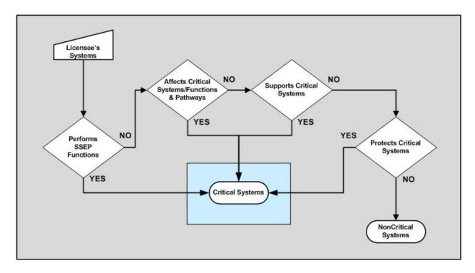
Figure 3 Evaluation process for determining critical systems
